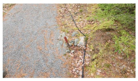
Image 9.3: Oriented NE- View of an Iron Property Bar and Wooden Stake Along the Southern Boundary of the Property.
