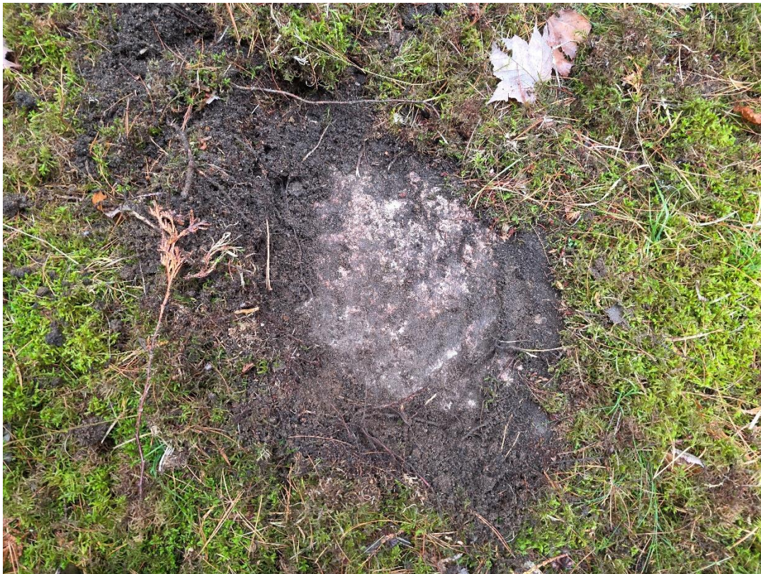
Image 9.10: Oriented SW- Shovel Test Showing Thin Soil Profile Above Bedrock.
